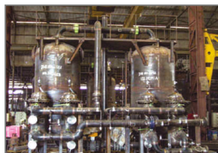
3 nos Air Dryer Unit Type : Heatless, Capacity : 13400 NM /hr For Paradeep Refinery project of IOCL
