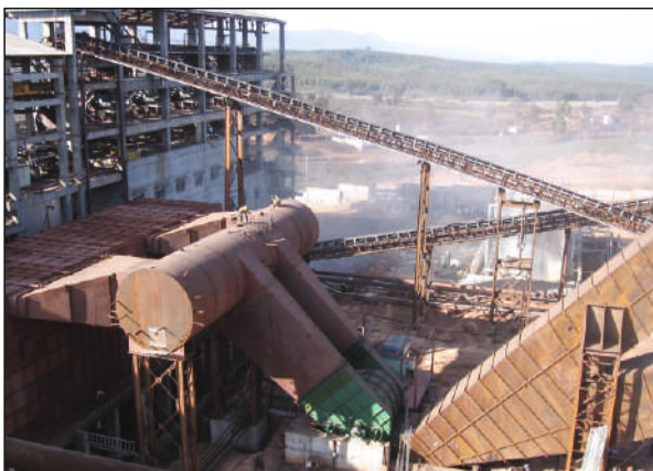
Rotary kiln, cooler & ABC / DSC equipment for sponge Iron plant
