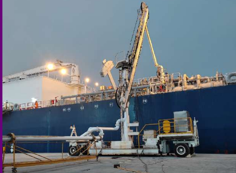
Trailer mounted marine unloading arm with jumper assembly for liquid ammonia services
