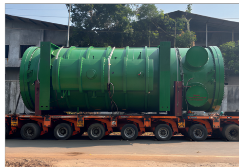
Surface Condenser for LMEL
